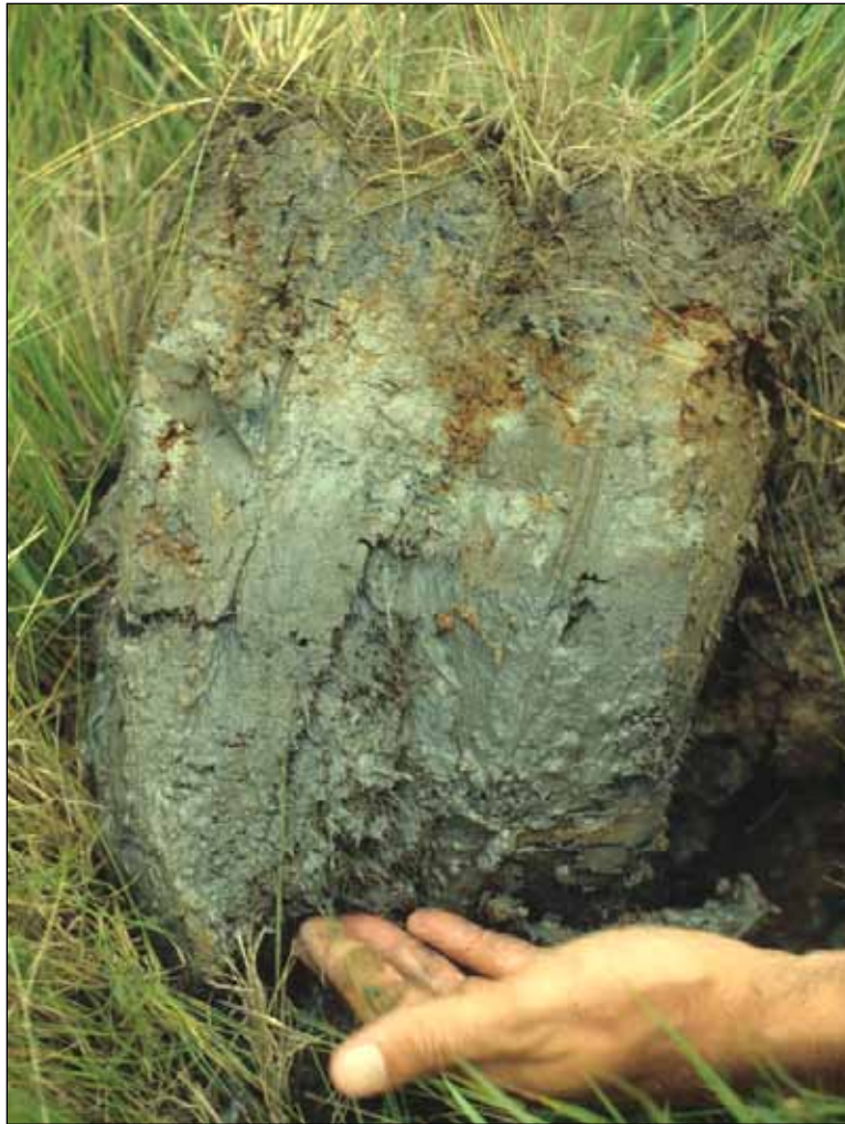
Figure 22. This soil has a gleyed matrix in the lowest layer, starting about 7 in. (18 cm) from the soil surface. The layer above the gleyed matrix has a depleted matrix.
