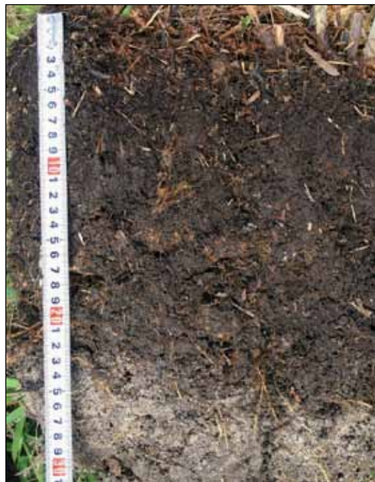
Figure 9. In this soil, the organic surface layer is about 9 in. (23 cm) thick. Scale is in centimeters.
